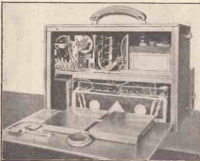
Rear view of the control box. The impulse motor is seen at the top left with the associated push-buttons (top centre). The flat boxes mounted on the inside of the opened lid contain tools, and a selection of spare parts.
