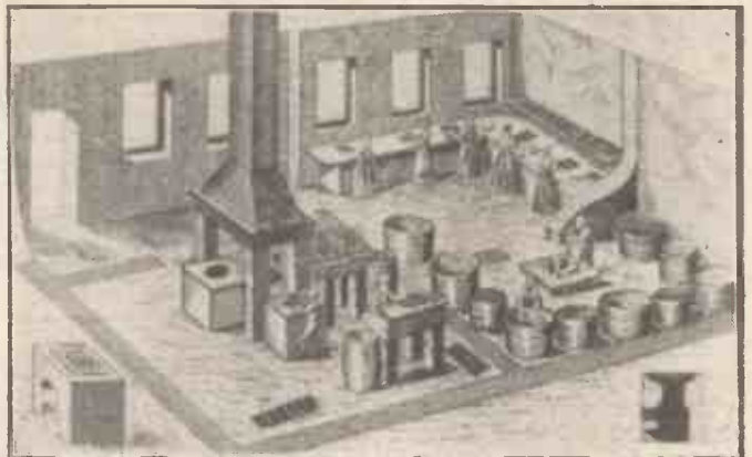
Making tinplate in 1714. The earliest illustration of the dipping process of tinplate manufacture.
