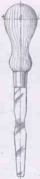
Fig. 1.—Screwdriver, showing application of leverage.
