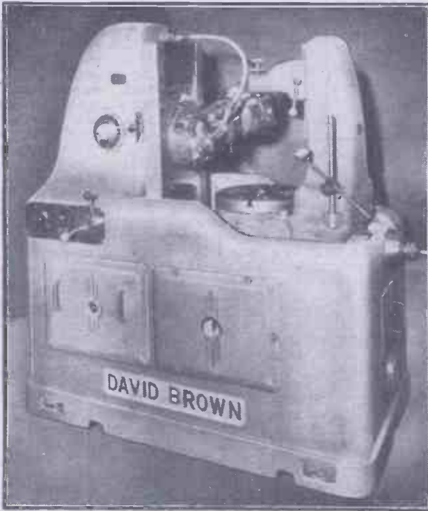
Fig. 1.—MT15 hobbing machine, by David Brown Machine Tools, Ltd., which made its first appearance at the Exhibition.
