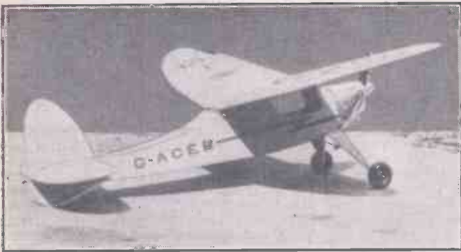
Fig. 13.—The author's small free-flight diesel-engined model "Meteorite" with span of 45½ in. can be converted to a control-line "Goat" in a few hours. The engine in this model is a 1 c.c. Frog diesel or a 1.3 c.c. Mills.
