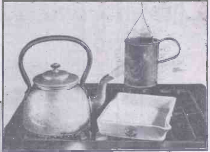
A simple experiment in vapour condensation. Steam from a kettle impinges against a suspended can of cold water. The tiny steam particles, being cooled, are immediately condensed into larger particles which collect on the colder surface of the can and which run off into the collecting dish below.
