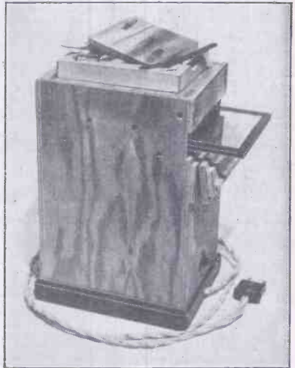
The completed printing box with the safelight partly inserted.
