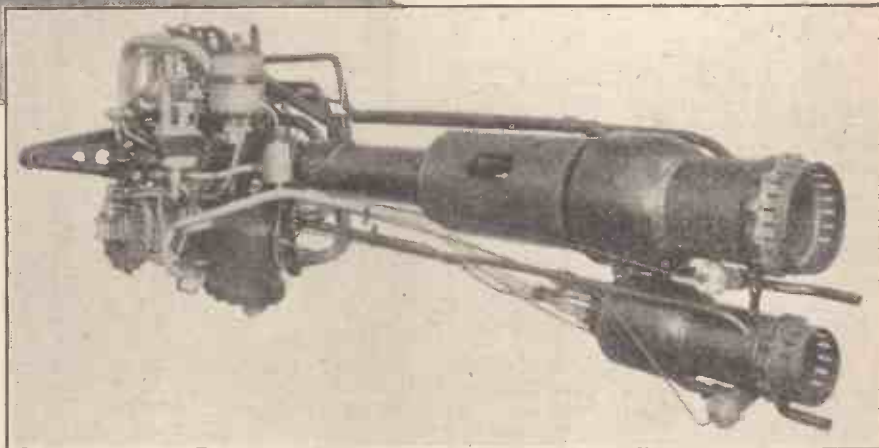
The Walter 109/509C developed for the Ju.263. Its main chamber produced a thrust ranging from 220 to 4,400lb., and an additional 880lb. constant was forthcoming from the smaller "cruising" chamber. (See PRACTICAL MECHANICS, Sept., 1946, p. 420.)
