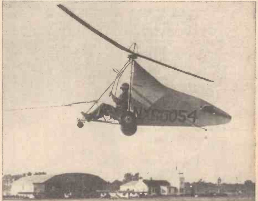
A wingless gyro-glider undergoing tests at the General Electric Test Centre in Schenectady, New York. I. B. Benson, one of the engineers responsible for its design, is at the controls.
