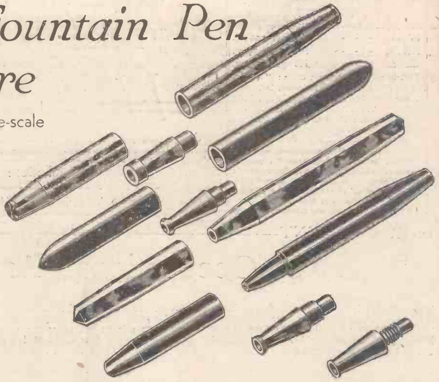
Fig. 1.—Barrels, caps, and pen sections are ground by the centreless process.
