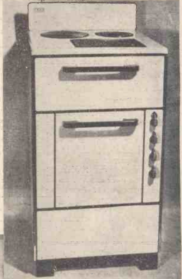
G.E.C. Standard Pressed Steel electric cooker. The oven is heated by tubular sheath wire elements and is thermostatically controlled. The drop-down door is of three panel rigid design and its fall is controlled by a patent braking arrangement.
