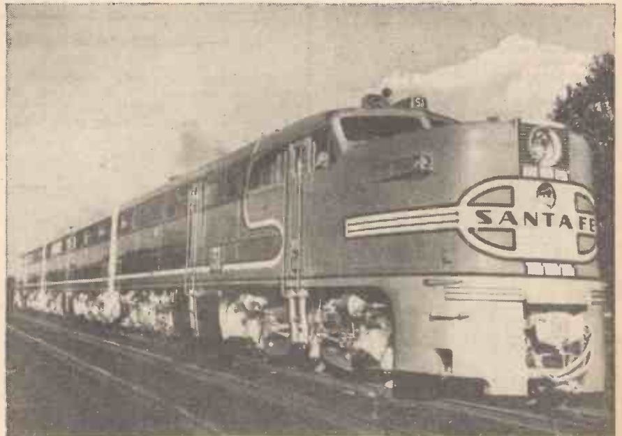
The 75,000th locomotive recently built by the American Locomotive Company. This 6,000 h.p. diesel-electric locomotive weighs 450 tons, and is capable of 120 miles per hour.
