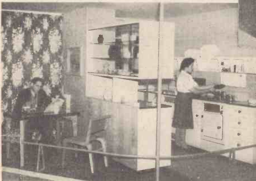
A kitchenette in a small flat where neither washing nor water-heating has to be done. It contains a prefabricated unit or package kitchen, a new product in aluminium and plastic, made up of nine units. A corner of the adjoining dining-room can also be seen in the illustration.
