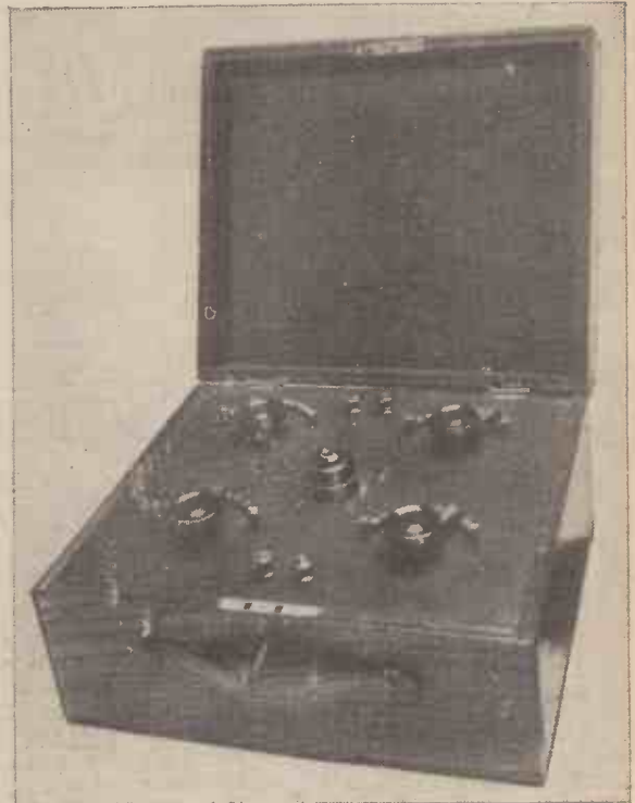
A modern laboratory resistance box for "introducing" ohms into a circuit. By a number of combined tappings it enables any number of ohms from 1 to 5,000 to be added to the resistance of an electrical circuit.
