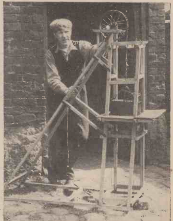
Mr. R. Barton, of Bolton, has invented a pit-cage safety device, designed to arrest the descent of a colliery cage in the event of the winding rope breaking. The illustration shows Mr. Barton with a pit-head model for demonstrating his safety device.
