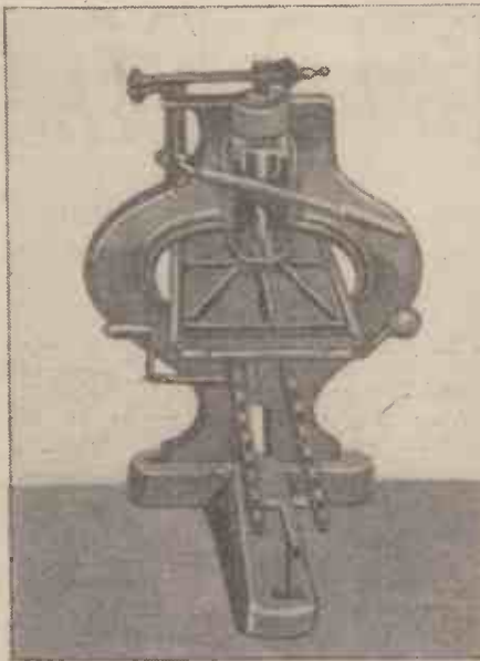
It revolutionised practical printing. The first iron printing press devised by Earl Stanhope in 1798.
