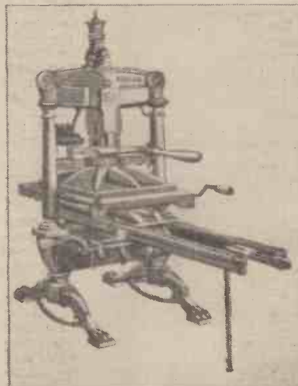
A mid-19th century iron printing press based on Stanhope's original invention.
