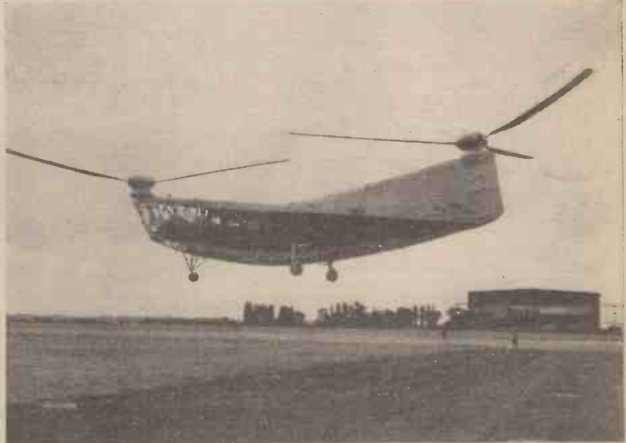
A new helicopter, the PV3, which will carry 12 passengers or the equivalent in cargo, has been constructed in Pennsylvania for the U.S. Navy. The machine is 48ft. long, 13ft. high, and has a rotor at each end. It can land within a 100ft. circle, and can be adapted for either land or water landing and take-offs. In the illustration the aircraft is taking off from the Navy Yard Airport for a test flight.
