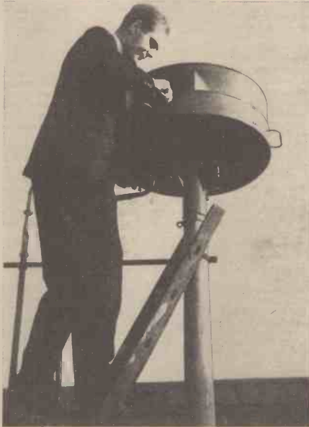
By means of radar the fog menace is banished from the sea. Fixed to the bridge deck of a ship is the "scanner"—a circular revolving reflector which sends out a continuous beam.
