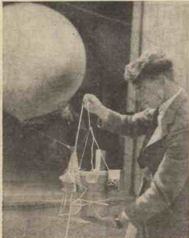
Fig. 40.—A small parachute is tied below the balloon which expands as it rises into the rarefied upper air. In the stratosphere, at a height of ten miles or more, the balloon bursts, and the apparatus floats down on the parachute.
