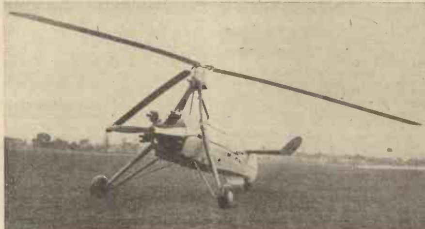
The autogiro, invented by Don Juan de la Cierva. This machine was the forerunner of the helicopter, but unlike the latter machine it cannot hover, as the rotor is not power-driven. Our illustration shows a "Direct Control" autogiro ready for a demonstration flight at the London Air Park, Hanworth, Middlesex, in April, 1933.
