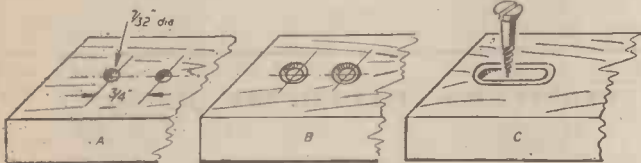
Fig. 9.—Method of screwing batten to the back of the drawing-board.
