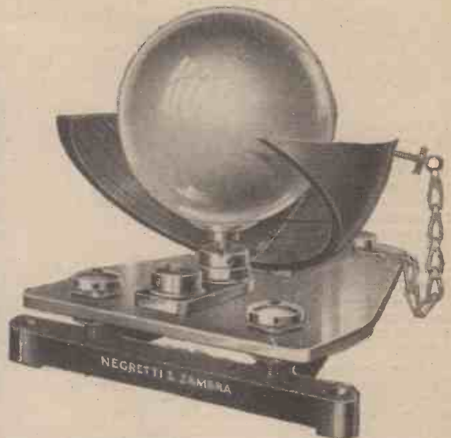
Fig. 24.—Sunshine recorder, Campbell Stokes pattern, for temperate latitudes. The sun's rays are focused upon prepared and printed cardboard strips. As the sun moves from east to west so is a tracing made on the strip.
