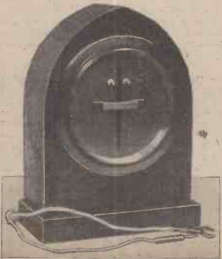
An early type of galvanometer based on Oersted's discovery. It was used for many years in the British Post Office.
