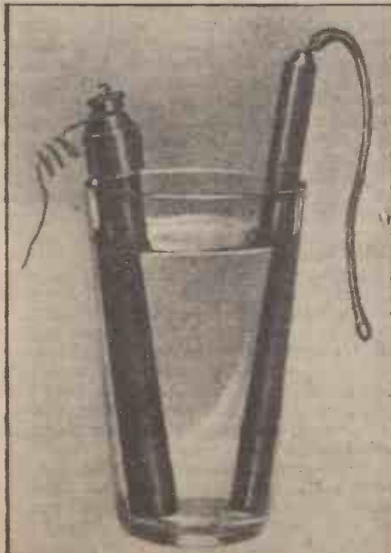
Another simple primary cell—zinc and carbon elements immersed in a solution of sal-ammoniac (ammonium chloride). From this was developed the well-known Leclanché battery.
