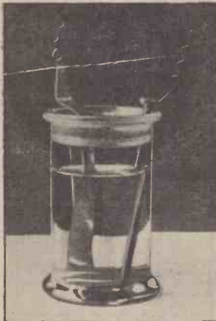
The simplest voltaic cell—electrodes of copper and zinc immersed in diluted sulphuric acid.
