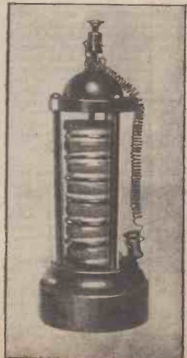
Volta's Pile, the world's first current generator.
