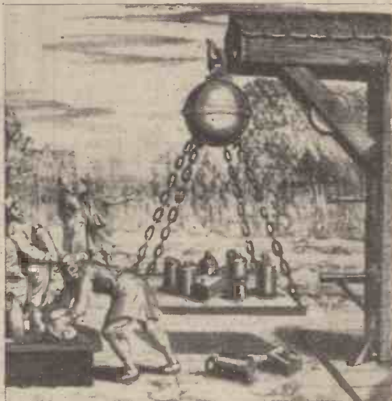
Fahrenheit observed the influence of atmospheric pressure on the boiling point of liquids. Here is a contemporary illustration depicting a demonstration of the effect of atmospheric pressure in holding together the two halves of a metal globe which has been exhausted of air. Despite loading with heavy weights, the lower half of the globe cannot be pulled away from the upper half, although if air were admitted to the globe its lower half would fall away at once.
