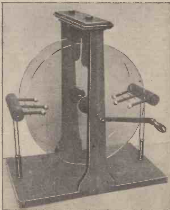
Original electrical machines are rare nowadays. Here is a recent photograph of an early machine constructed on the disc principle originated by Jesse Ramsden. It is still in working order.
