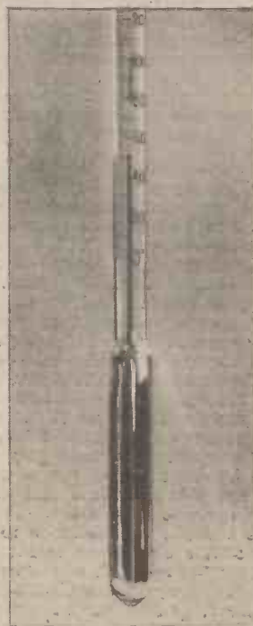
The lower end of a mercury thermometer, showing the cylindrical bulb, due to Gabriel Fahrenheit.
