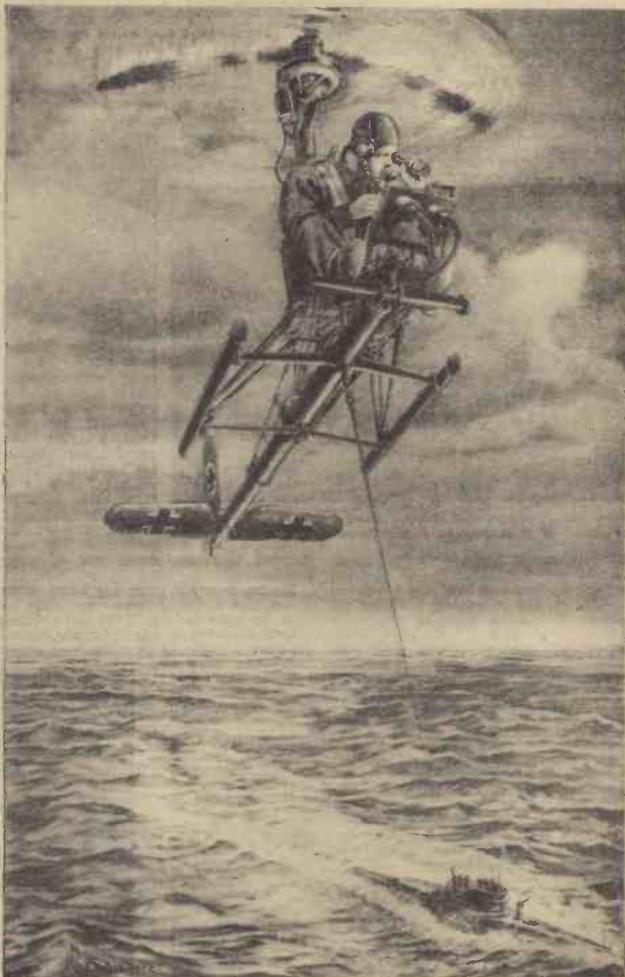
This midget autogyro is described by the Germans as the new eye of the U-boat. The machine is housed in a pressure-safe container in the submarine, and rises in the air when the U-boat is operating in the open seas. The propeller is driven by the forward movement of the U-boat, to which the machine is connected by a wire rope. The autogyro can operate up to 1,000 feet.
