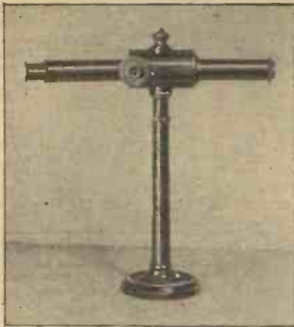
The spectroscope, an instrument by means of which a beam of light is split up into its components.
