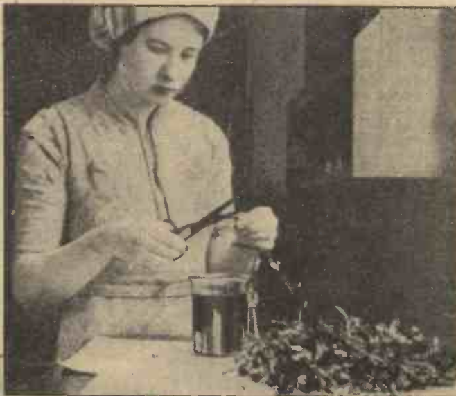
Cutting up the seaweed into small pieces for extraction with sodium carbonate solution.
