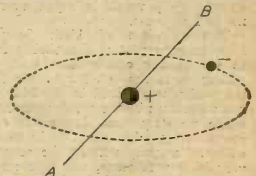
Diagrammatic illustration of an electron revolving in its orbit around the positively charged nucleus of an atom. The whole arrangement constitutes an effective gyroscope, which causes the atom, as a whole, to spin on its axis AB, and thus to set up fields of force which are supposed to give rise to magnetic effects.
