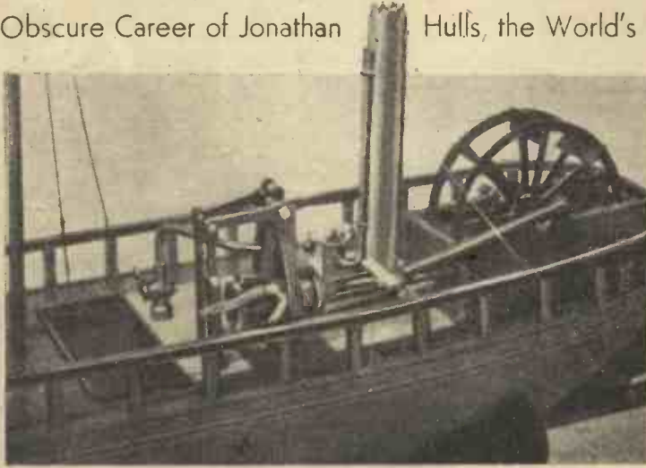
A close-up of the engine of Symington's steamboat, "Charlotte Dundas" (1801.) (From a Science Museum model.)
