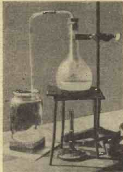
Laboratory apparatus for the preparation of chlorine gas from hydrochloric acid and manganese dioxide.
