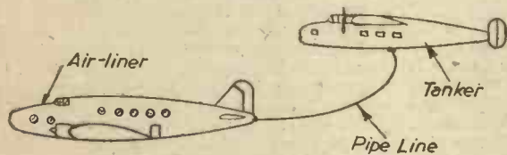
Fig. 1.—Method of refuelling an air-liner in flight.
