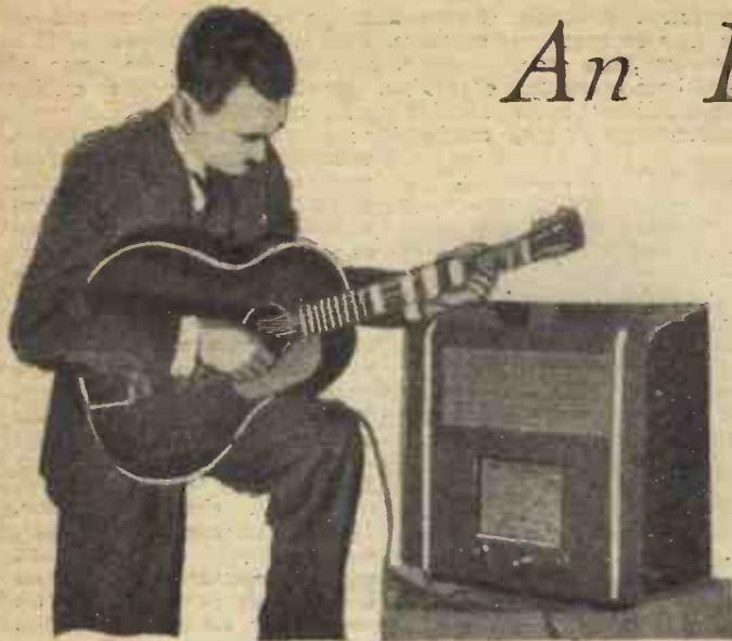
The completed "electric" guitar being used in conjunction with the pick-up circuit of a radio receiver.
