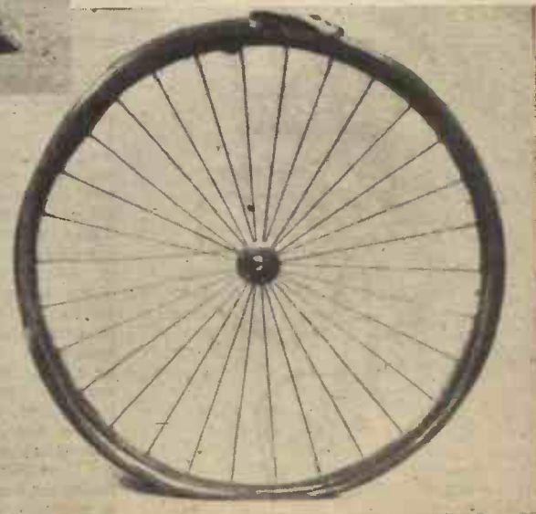
The invention which "made" the rubber trade—J. B. Dunlop's first pneumatic tyre.
