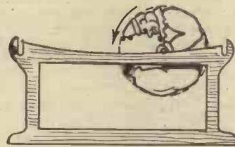
Fig. 7.—When the lower end of the string is pulled the windmill will rotate at a rapid rate, whistling whilst doing so. It will also re-wind itself.
