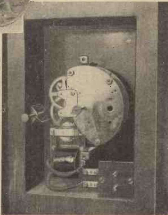
Fig. 2.—Showing how the motor is mounted in the clock case.
