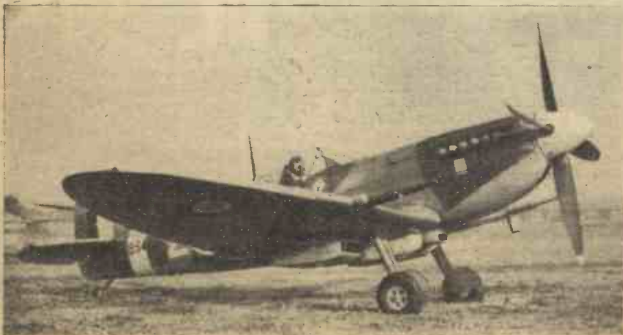
An improved Spitfire, showing the slightly longer nose, with four-bladed propeller and multiple outside exhausts. The two cannon guns can be seen on the wings.
