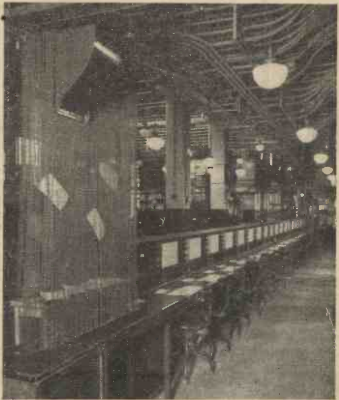
The conveyor band system, showing the chain-guarded drop, and slow-moving band. Note the pneumatic tubes overhead. (By the courtesy of the Postmaster-General.)
