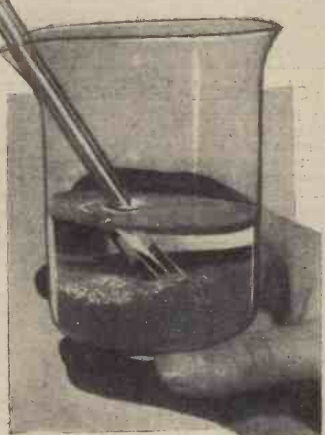
Illustrating the nature of a saturated solution. A beaker containing water and crystals of a chemical salt. The water has dissolved a maximum amount of the crystals, and it will not dissolve more. The resulting clear solution is therefore "saturated."
