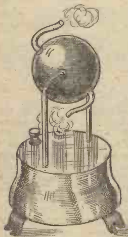
Hero's "æolipile" engine, 150 B.C. The base is hollow and constitutes the boiler.
