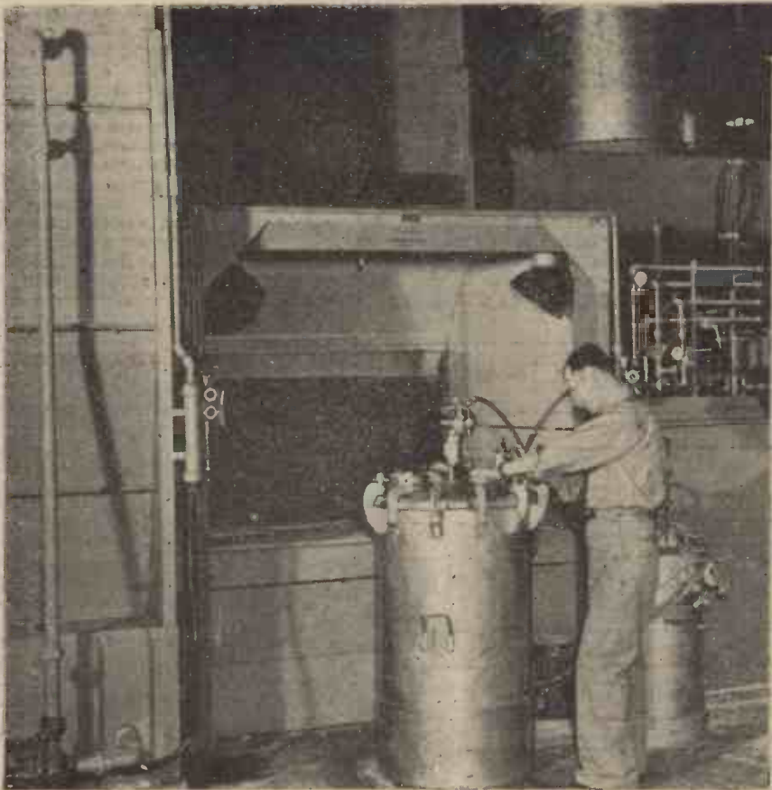
Fine paint spray and fumes are sucked up through a ventilator stack, screened by a "waterfall," which serves as a filter, removing the highly-inflammable paint "dust" from the air. In the foreground is one of the pressure vats where the paint, constantly agitated, is kept. Tubes from the vat feed the paint to the overhead sprays.
