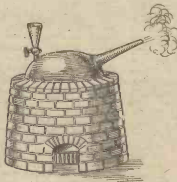
Savery's spherical boiler, 1698.
