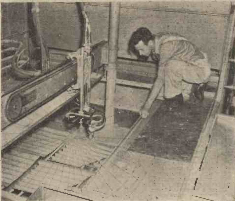
Whipping across the endless procession of small parts are the automatic spray guns, spreading an even coat of corrosion-resistant paint on the pieces soon to be included in the construction of a Martin bomber. Two such units comprise vital phases in the process.
