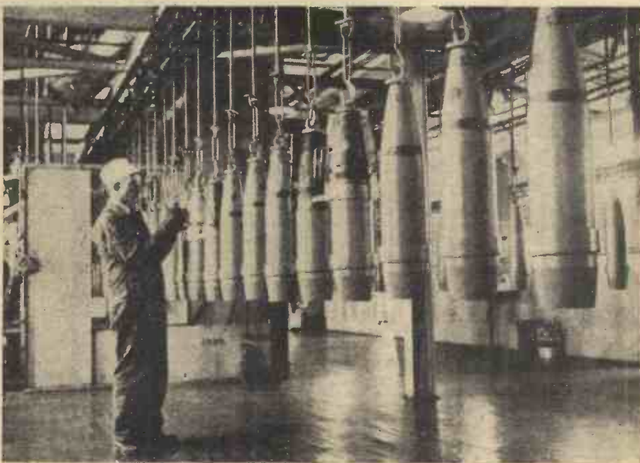
Slowly revolving on the endless trolley, these huge shells are borne into the painting room at one of Canada's munitions factories. Quickly, a painter sprays the shell from top to bottom with an air-pressure gun, and the trolley carries it along to the next operation.
