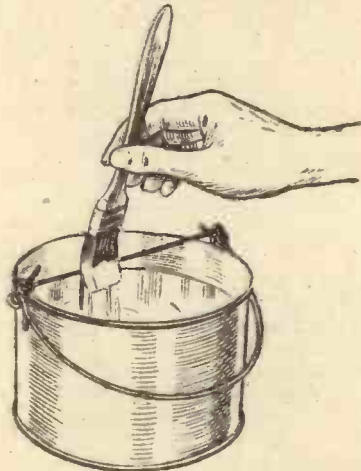
Fig. 2.—A piece of string tied across a paint can for removing superfluous paint from the brush.
