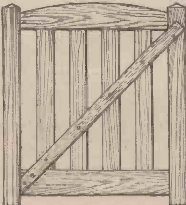
Fig. 4. Using a diagonal bracing piece for a sagging gate.
