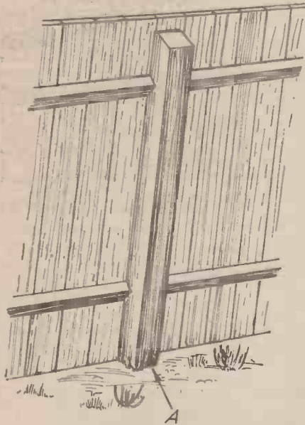
Fig. 1. Part of a close-boarded fence, showing where rot usually starts.
