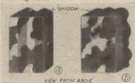
(a) Shows shadow cast by normal building. Where this cannot be merged into general surroundings a camouflage superstructure may be used to break up outline and give shadow, as at (b).
