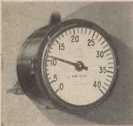
Fig. 9. Indicating Ring Balance meter.
