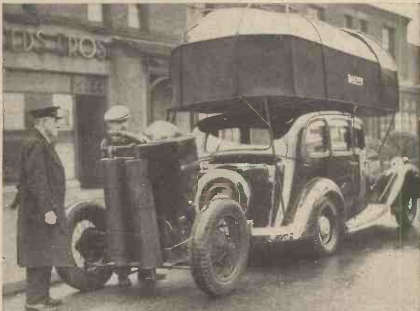
A private car with a gas bag and trailer for supplying coal gas. Mr. Barton, the inventor of this gas system, which was used during the last war, is seen on the extreme left.
