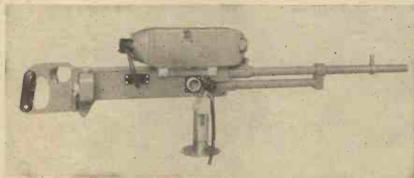
Fig. 11. Cine camera gun G.42B, on type 29 mounting (fixed).
