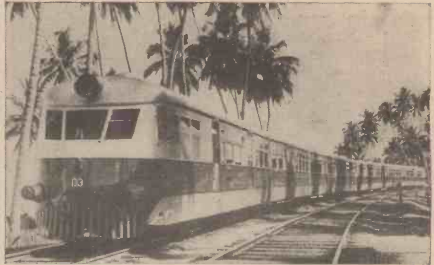
Fig. 3. An eight-coach (two four-coach units) "English Electric" Diesel-electric articulated train in service on the Ceylon Government Railways.
