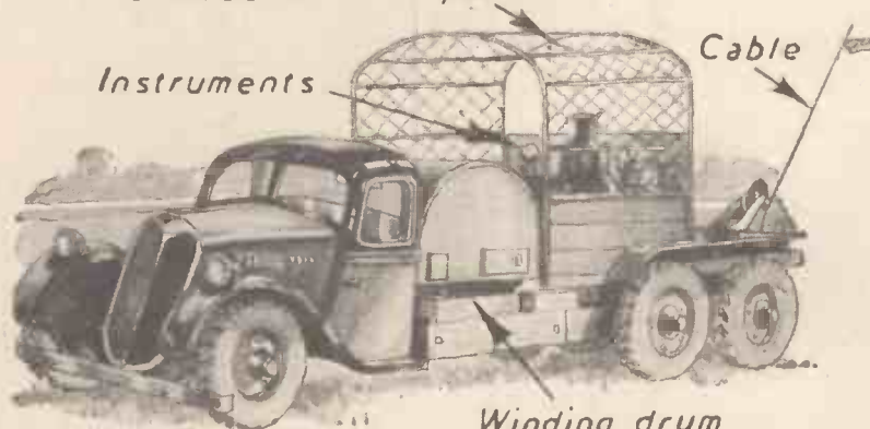
Details of the lorry for carrying, raising and lowering the balloon
