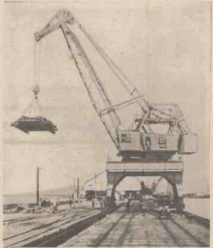
Fig 5.—An example of the wharf type of jib crane. By means of the folding lever on the jib head, the movement of the jib inwards and outwards can be attained without lifting and lowering the load. Thus the load maintains a horizontal path, hence the name given to this type—the level luffing jib crane.
