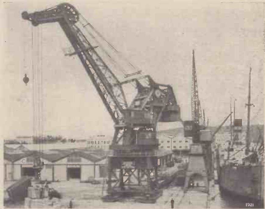
Fig. 3.—An 80-ton Babcock crane installed in South Africa.
