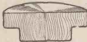
An example of well-controlled grain flow in a gear wheel blank; this blank would produce a quiet gear.
