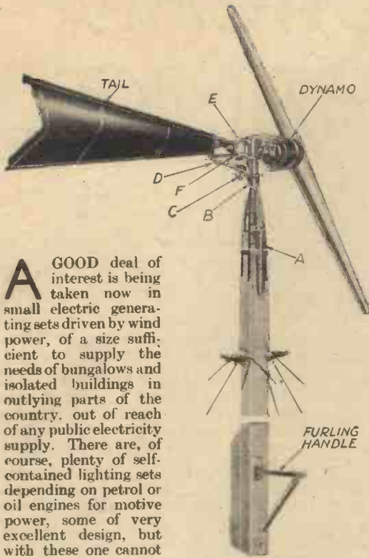
Fig. 1.—A commercial set which relies principally on the self-governing properties of the dynamo, aided by a furling action of the wind-motor tail
