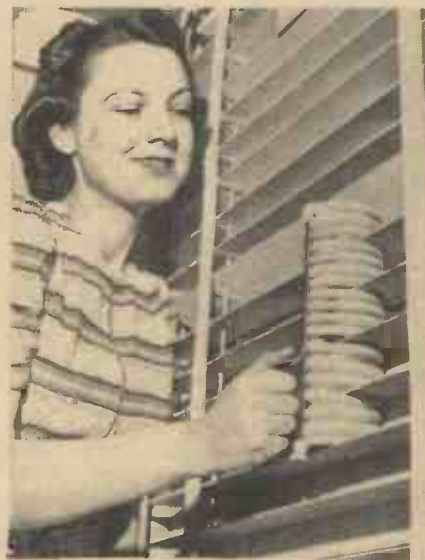
A venetian blind mop, invented by Kenneth Wade, of New York. It cleans five slots at one clip
