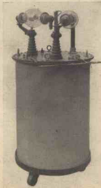
Fig. 2.—The specially developed E.H.T. unit which furnishes the anode volts essential for the proper operation of the C.R. tube.
