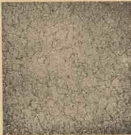
× 450 High-speed steel correctly hardened.
