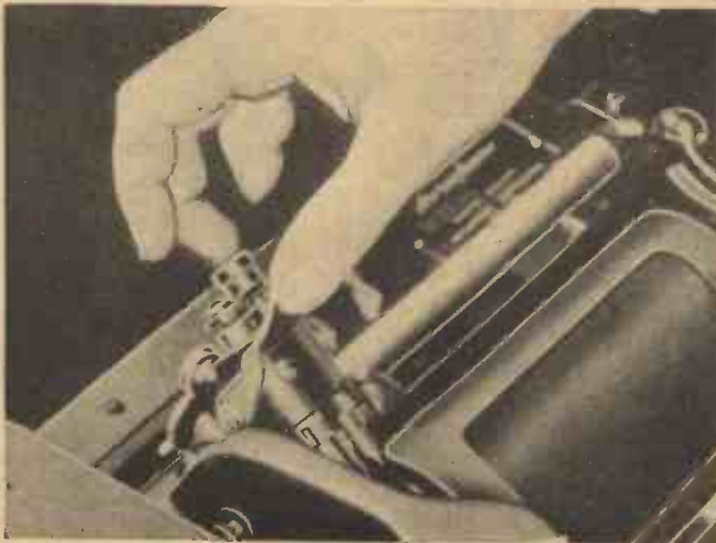
Fig. 11.—Setting the shaver blade.
