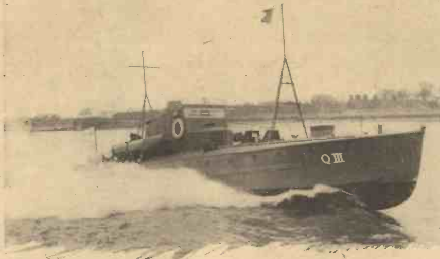
The new Thornycroft motor torpedo boat which reached a speed of 41 knots in her trials
