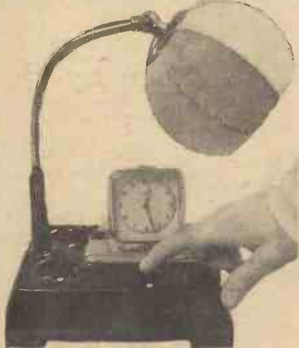
A combined alarm clock and lamp. When the alarm goes off the lamp lights up.
