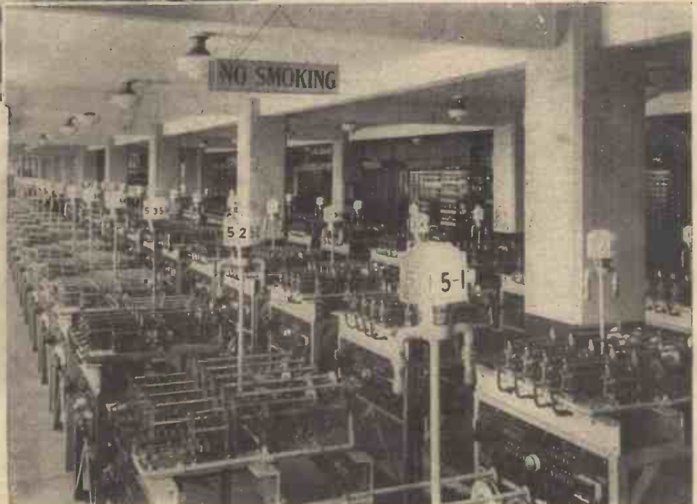
(Right) General view of main adding machine. Each adding unit is complete with its own motor drive.
