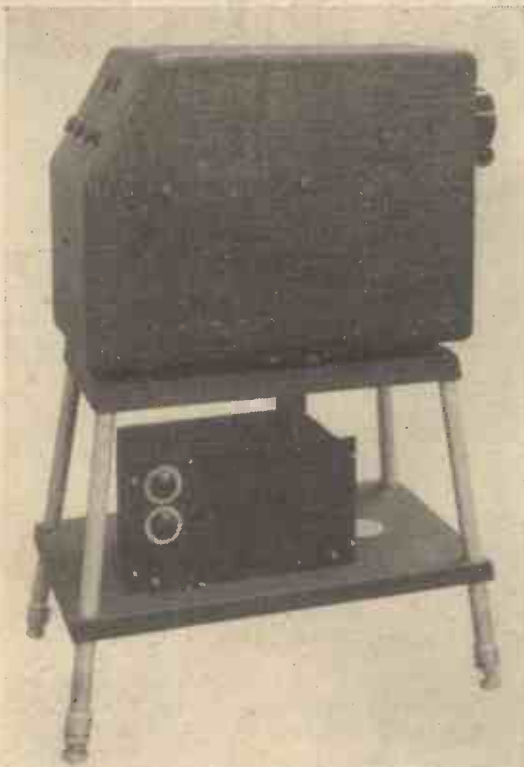
Fig. 1.—The projector unit which houses the C.R. tube, time-base and amplifier equipment.
