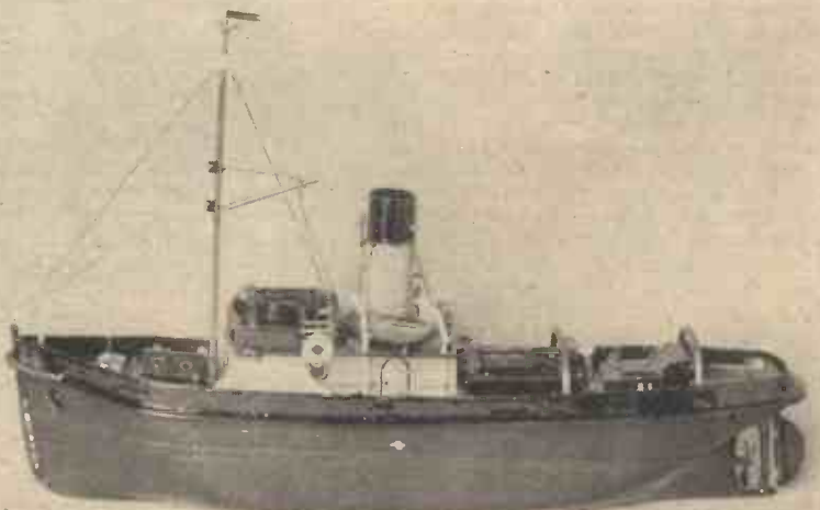
A model steam tug made by Philip Scott-Martin. It measures 9½ in. long and is equipped with a working model engine of only ½ in. bore and stroke, made by the Editor of this journal.
