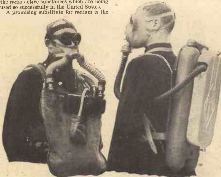
The new compressed air apparatus (right), compared with the old oxygen type (left) at a demonstration at the Fire Brigade Headquarters in London.
