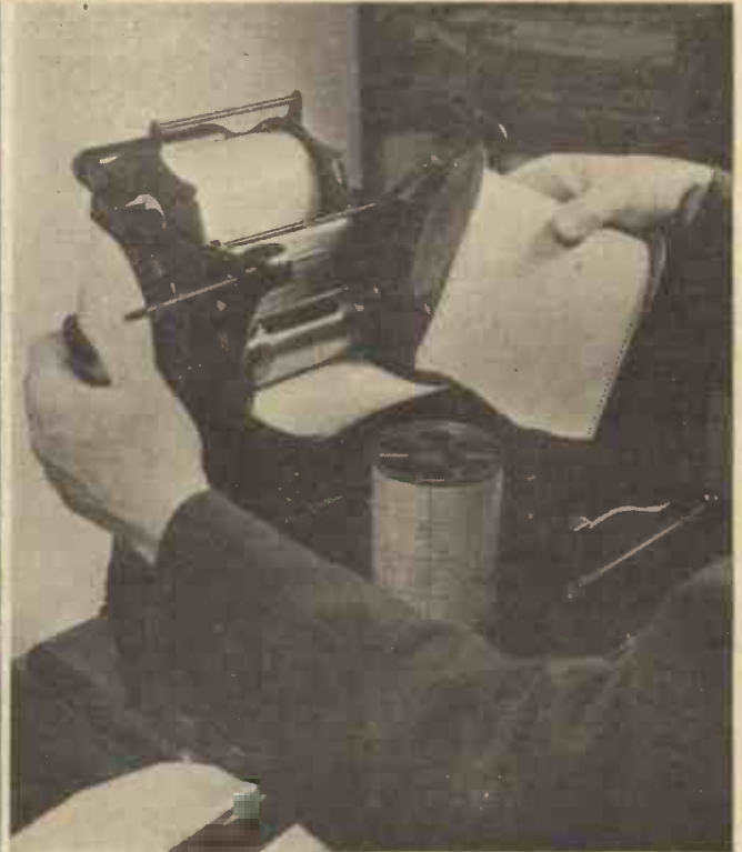
(Left) The Monotype keyboard. Notice the great range of different character keys including independent italic, small caps and bold alphabets. (Right) A paper ribbon, perforated by depressing the keys of a Monotype keyboard, forms a permanent record of the setting. Here the operator is just taking off a perforated spool, containing part of the record of 4 hours' tapping, and this will be transferred to an independent caster.
