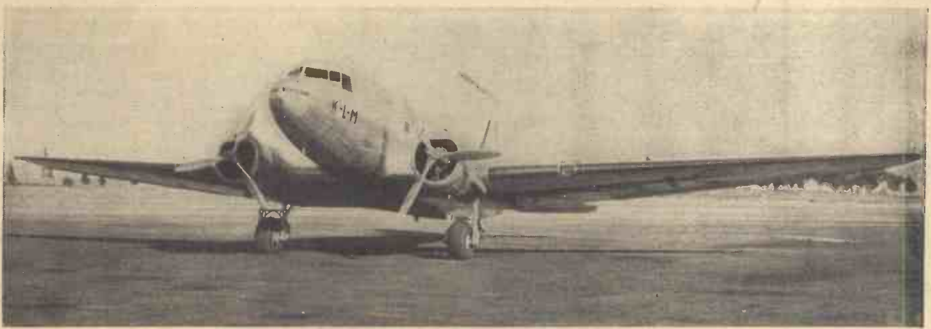
The first airplane to be exported from the United States equipped with the new Wright G-100 Series Cyclone engines rated at 1,100 h.p. for take-off—a Douglas 21-passenger DC-3 transport, first of a new fleet of similar ships to be placed in operation by K.L.M. between London and the Dutch East Indies.
