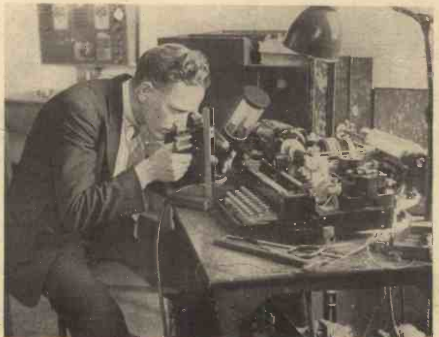
Teleprinter transmission contacts undergoing micro-examination at Dollis Hill.
