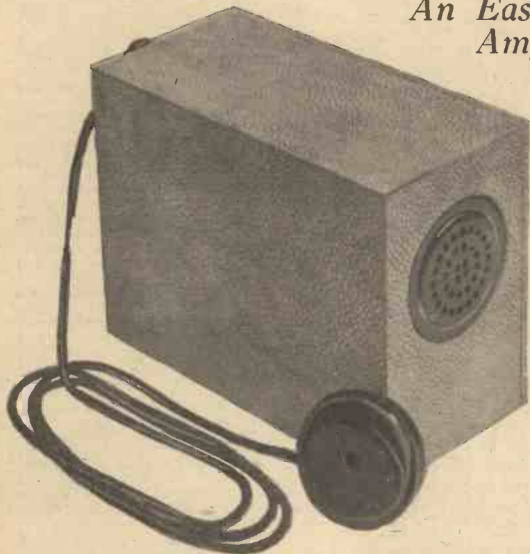
Showing the neat and attractive case of the completed deaf aid.
