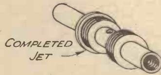
CUT THREAD ON JET BEFORE CLEARING CENTRE
