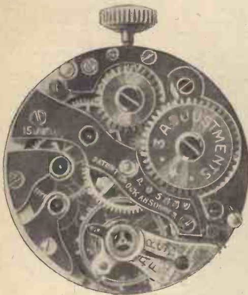
Fig. 1.—A modern Swiss lever movement of the popular 10½ ligne size
