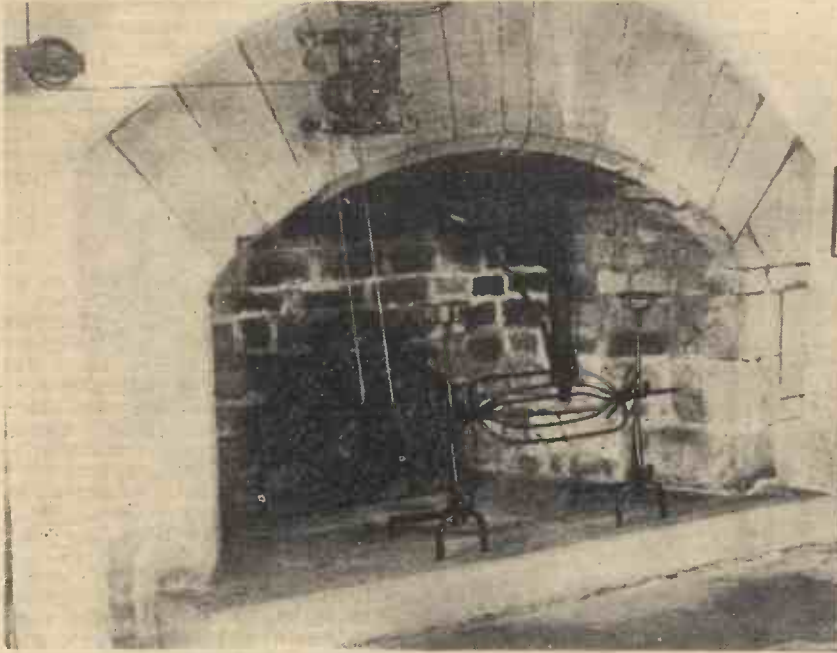
A fine example of the old English weightdriven "split-clock" device for slowly revolving a roasting spit before the fire. It is supposed to be the invention of Leonardo da Vinci.
