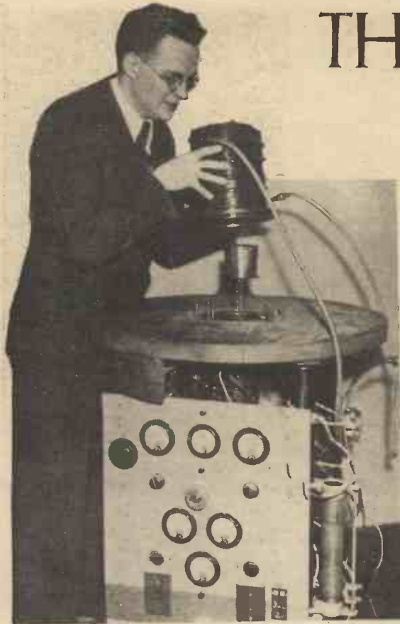
A new "Electron Bombardment" furnace, permitting scientists to heat metals up to temperatures of about 4,500 degrees Fahrenheit, almost half the temperature of the sun, has been perfected by Dr. Ralph R. Hultgren, Harvard metallurgist, who is shown here placing a vacuum cover over the furnace.
