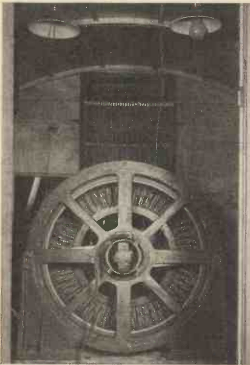
Fig. 1.—The commutator and back of the lamp screen used for the big screen demonstration in 1930
