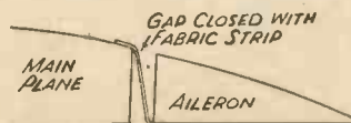
Fig. 10.—A strip of fabric connecting the top surface of the wing and the undersurface of the aileron.
