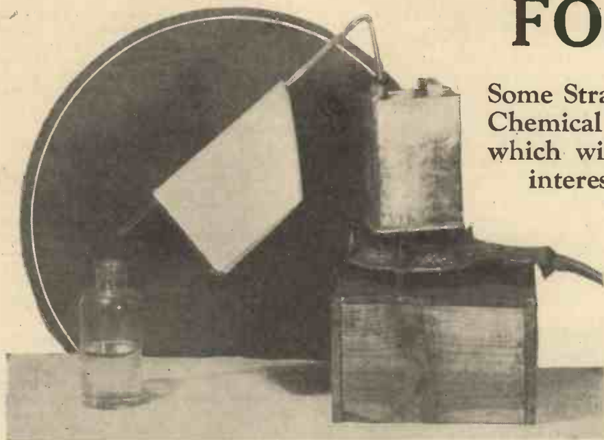
A simple form of distilling apparatus made from an old tin and a piece of glass tubing. It is suitable for many varieties of chemical distillations.
