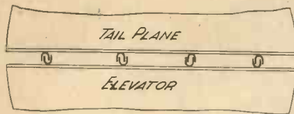
Fig. 6. (left).—Details of the hinges. Fig. 8 (right).—The rudder lever.
