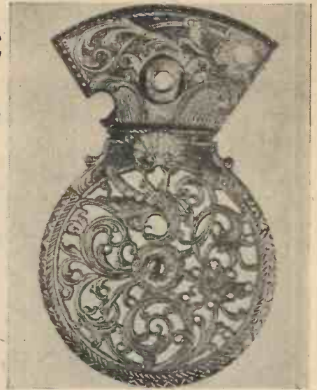
A chased "cock" from an old verge watch (original \frac{3}{4} -in. in length).
