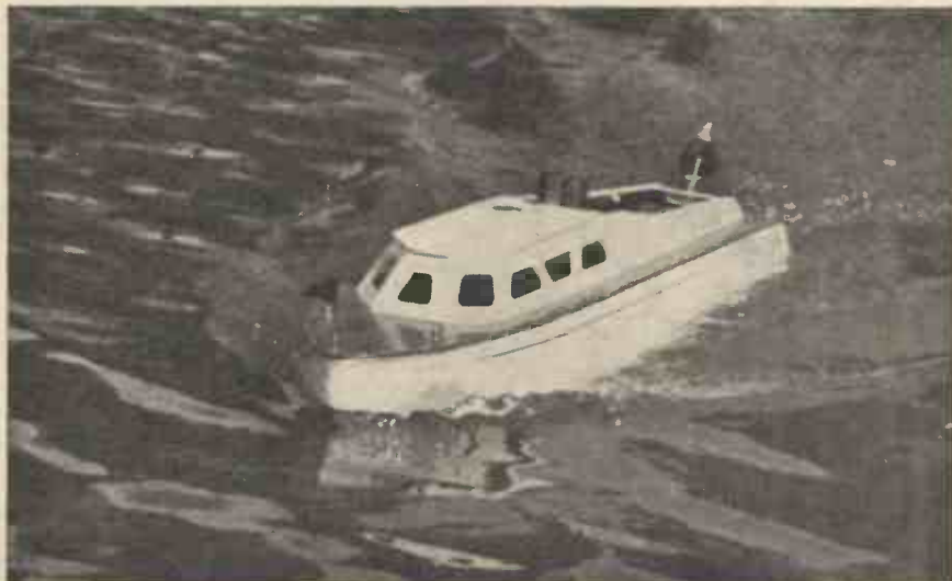
A model metre racing motor boat, "Streamline," doing 8 knots under test. This model was made up and described in "Practical Mechanics" last year, the parts being obtainable from Messrs. Bassett-Lowke, Ltd.
