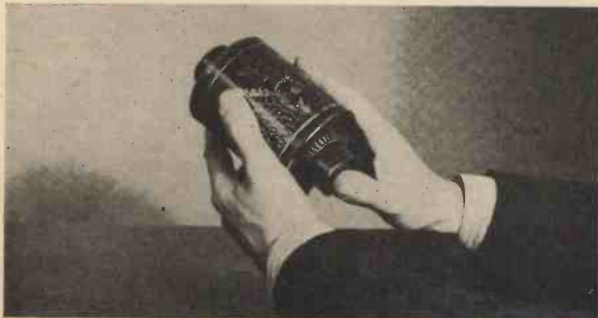
Fig. 14.—A changing canister. This photograph shows how the double-ended inner canister is pushed through its outer casing, thus making the compartment in the opposite end of it available.
