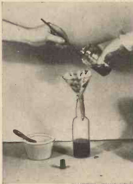
Making Indian ink. The ground-up mixture of lampblack and gum arabic solution being filtered through cotton wool.
