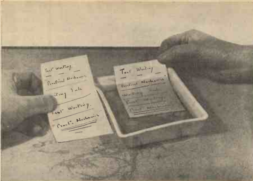
The "water immersion" test for the permanency and waterproof nature of writing ink. All Indian and iron-containing inks should be made to undergo this test.
