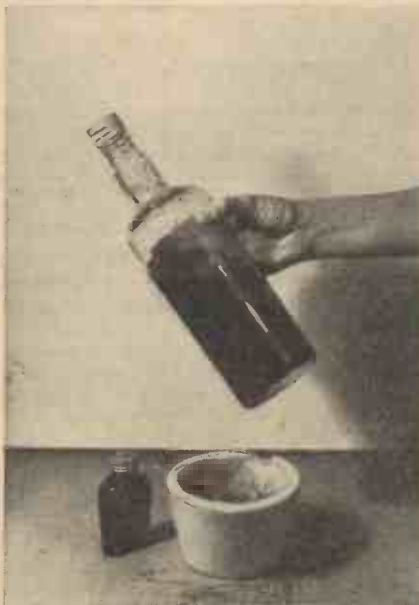
In the production of "old-fashioned" black writing inks, the ingredients must be well shaken up in a bottle every day for a fortnight.
