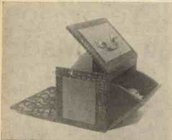
Fig. 1.—An exposed view, showing the secret V-shaped compartment. When the compartment is swung inside the box, the back of it becomes the panel on the back of the box.
