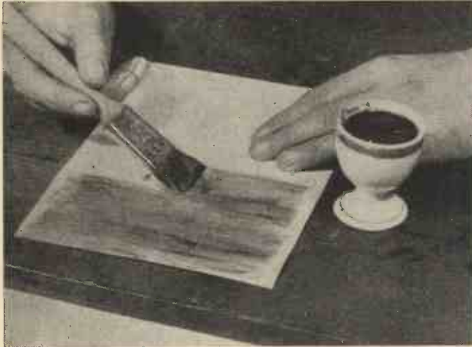
Pigmenting the paper. Note the flat brush employed.
