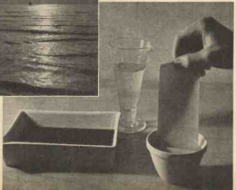
(Above) A fine piece of photographic work and (Right) After being desensitised, the film can be handled in the light of a candle, making it easy to see how development is progressing.
