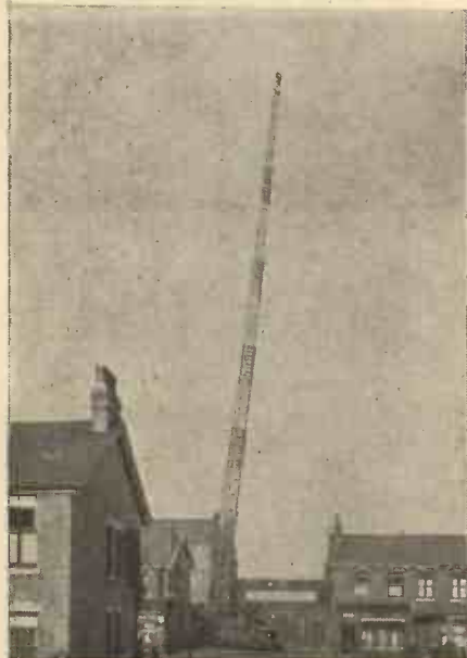
The 180 ft. Leyland fire escape, which is the highest in the world.
