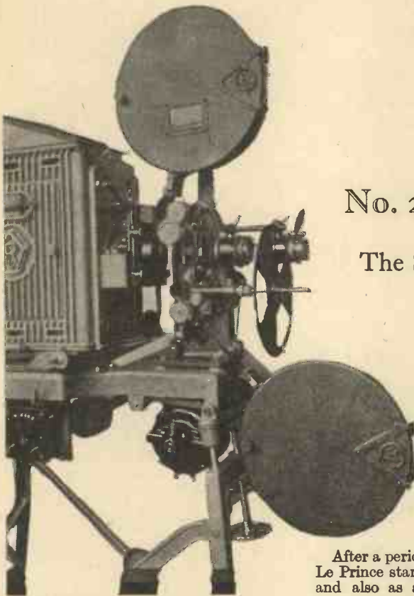
A modern cinematograph projector for silent films made by Ross, Ltd.
