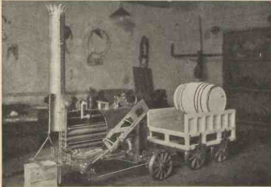
A view of the partly finished 1 1/2-in. to the foot scale model of the Rocket and parts, in the course of construction.
