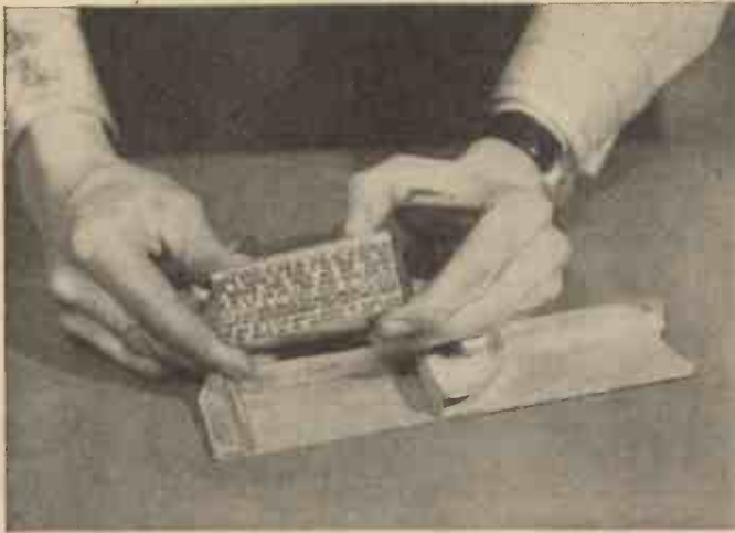
Removing a stickful of type from the stick.
