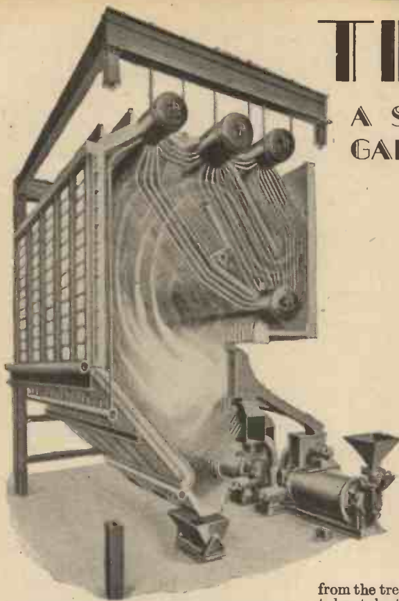
The arrangement of a pulverised fuel fired water-tube boiler. The grid arrangement of the burners can be clearly seen, and the method of lining the furnace on every side with water tubes is shown. A bogie truck under the throat of the furnace stands ready to take delivery of the ash of the burnt fuel.
