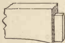
Fig. 8.—How the shaped rail is tenoned into the side.
