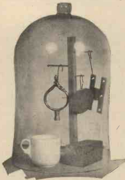
Copper and brass objects moistened with vinegar and suspended in an atmosphere containing carbon dioxide gas evolved from a soda solution contained in the cup.
