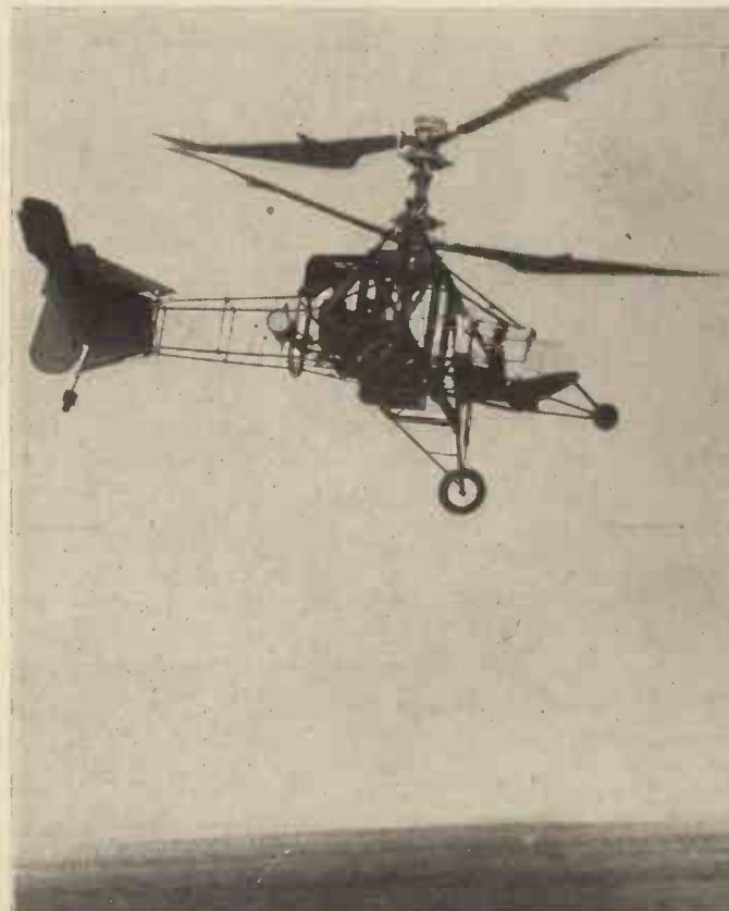
The Breguet gyroplane, fitted with a 300 h.p. Hispano-Suiza engine, which won the French Air Ministry prize for "hovering." It was stationary in the air for more than ten minutes.
