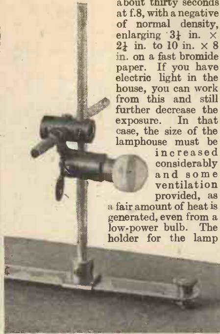
Fig. 5.—The holder for the lamp.
