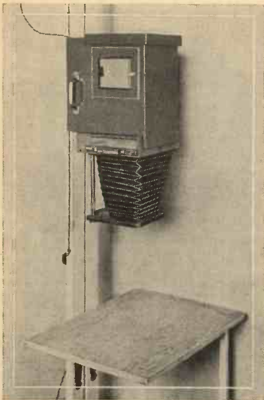
Fig. 1.—The finished vertical enlarger.
