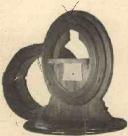
The original galvanometer used by Joule in his experiments on the heating effects of electricity.
