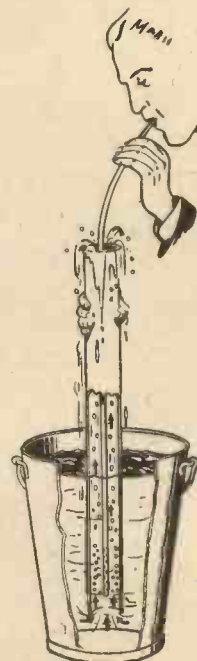
Fig. 4.—Demonstrating the air-lift method of pumping water.
