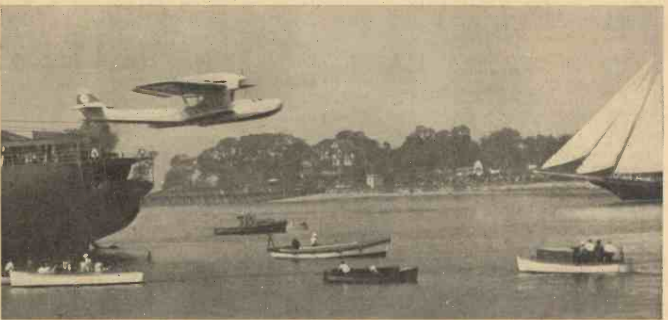
The giant German flying-boat "Zephyr" is shown leaving the catapult aboard the steamer Schwabenland, on a test hop. The "Zephyr" with its sister-ship "Aeolus" are being used on tests over a proposed Trans-atlantic commercial air route, with the Schwabenland acting as a floating, mid-ocean airport. The above illustration, gives an excellent example of the advances in transportation with the huge flying-boat leaving the stern of the steamship.
