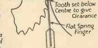
Fig. 13.—Details of the spring tooth-rest.
