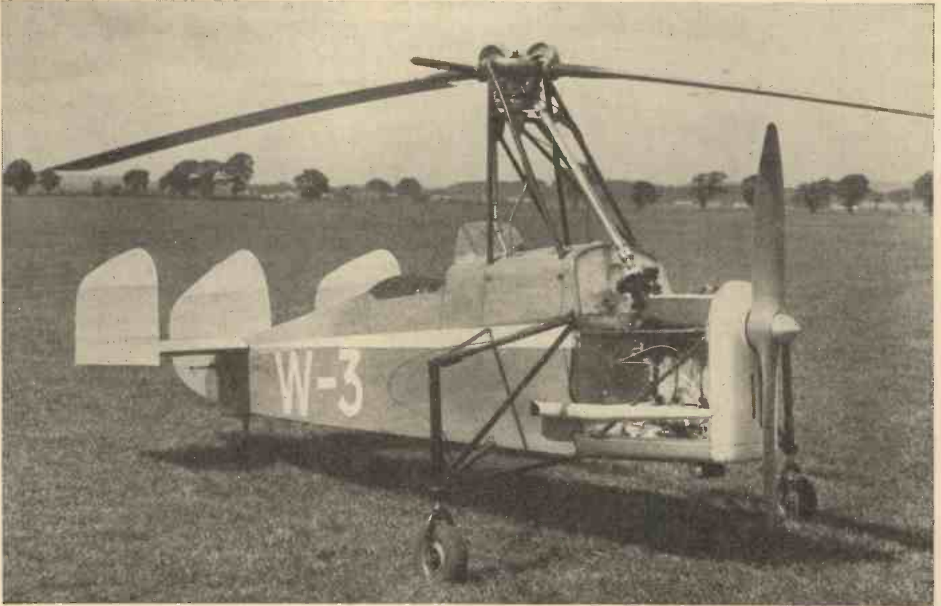
Fig. 1.—The latest type of "Direct Take-Off" autogiro. It is fitted with a two-bladed rotor, the blades of which are set to zero incidence while being speeded up before the take-off.
