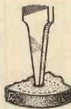
Fig. 12.—Boring a hole in a broken wheel with the tang of a file.
