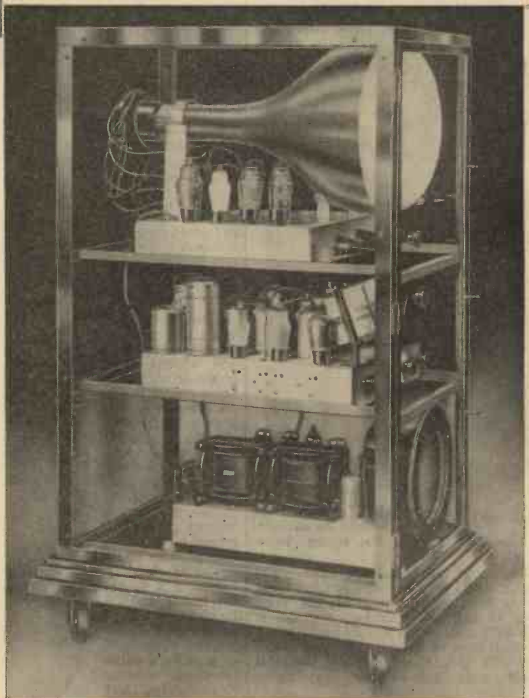
The arrangement of the tube and chassis of the model shown above.
