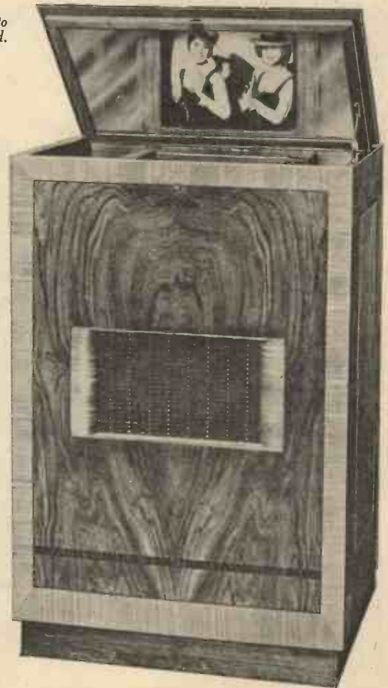
The Marconiphone Model 701 has a reflector to enable the vertical cathode-ray tube to be viewed.
