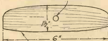
Fig. 36.—The rowing chock, made from oak 1 1/2 in. square.
