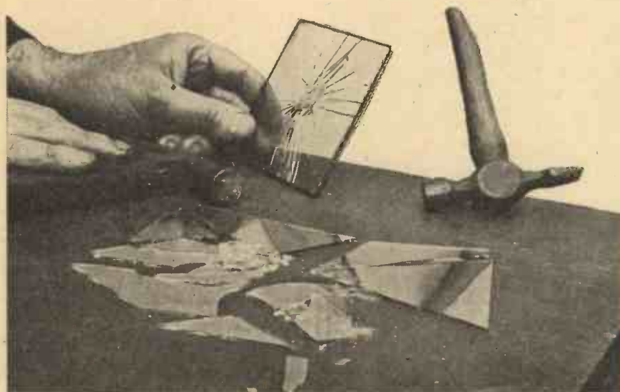
This picture clearly shows the difference between ordinary and safety-glass.
