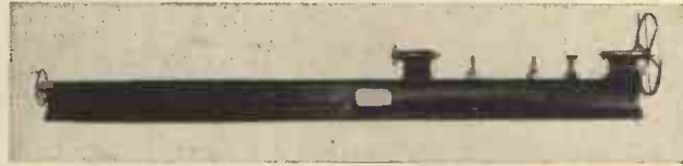
A micrometer screw-gauging machine made by Whitworth. It is one of the three instruments of this type which he constructed.
