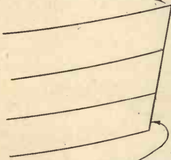
Fig. 29.—The surplus top of the stem post cut flush with the chines.
