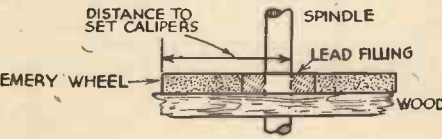
Fig. 1.—Method of mounting emery wheels.
