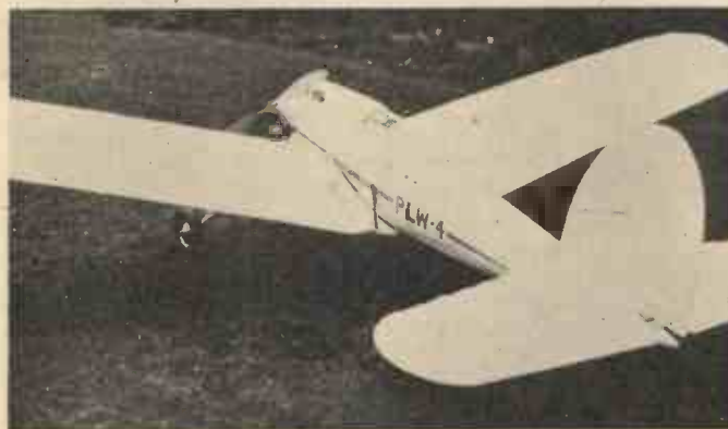
Fig. 15.—Rear view. Note the position of the clock, and also rear retaining elastic bands for the low wing.
