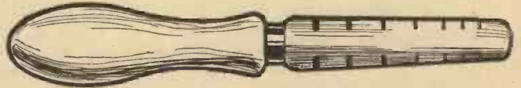
Fig. 7.—A simple saw-set consisting of a strip of steel with notches of different widths. One of these is used to grip the teeth when bending.
