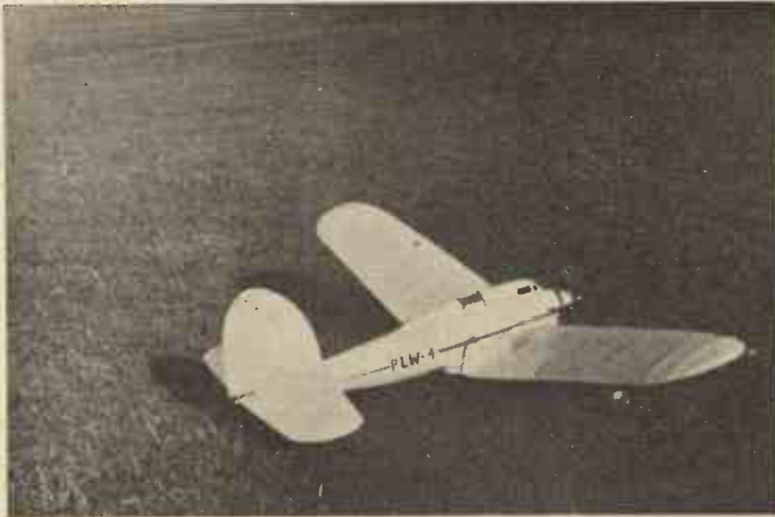
Fig. 1.—The petrol-driven low-wing model P.L.W.4.
