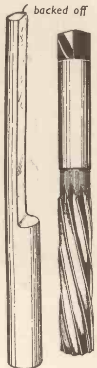
Figs. 6 & 7.—(Left) A reamer made in the form of a dee bit, and (right) a fluted reamer.
