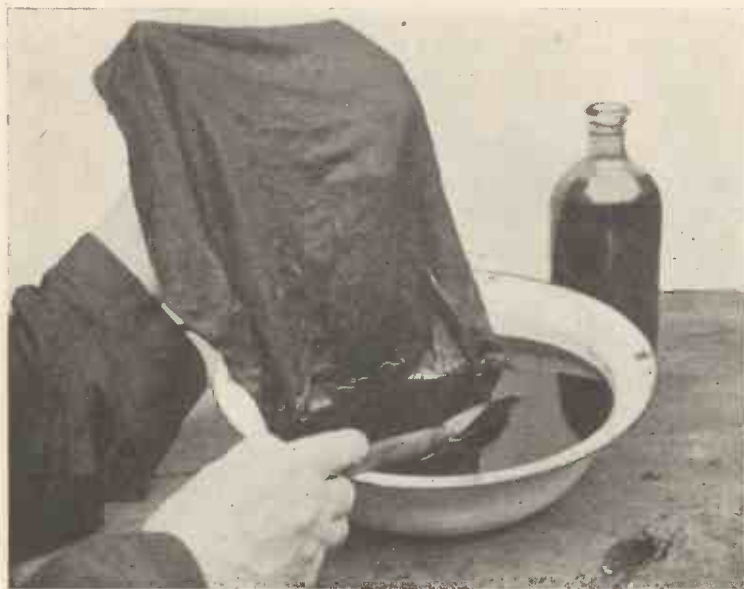
Woolen material after being mordanted with an iron salt, being entered into the cold dye bath.
