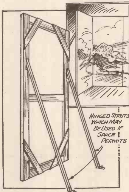
Fig. 6.—A useful scenery frame. The number of these required will depend on the type of set required and the size of the stage.
