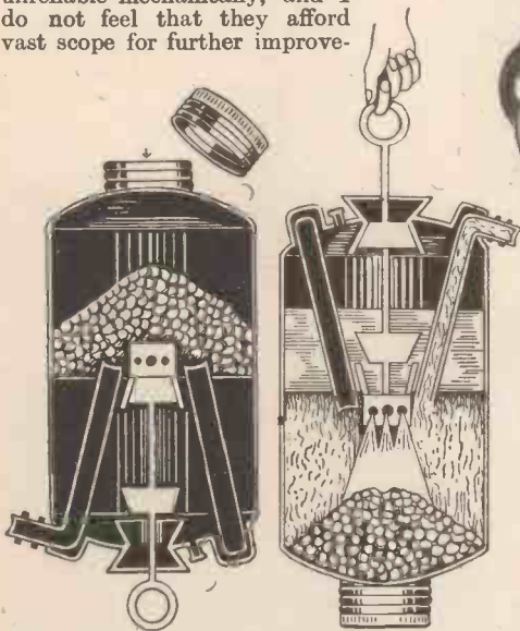
The container is first filled with carbide, as shown on the left, and the latter is then covered with dry ice. When inverted, as on the right, and water is allowed to drip on to the ice and carbide, a non-inflammable gas is given off at high pressure.
