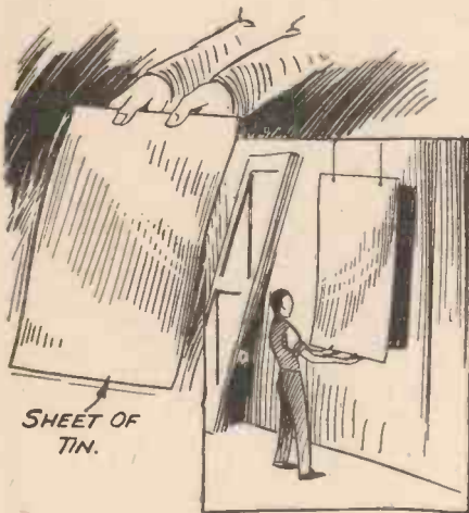
Fig. 1.—How the noise of thunder is produced.
