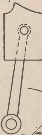
Fig. 4.—Drill the prop. boss for the bolts in such a position that the blades are making an angle of 45° with the vertical centre line of the engine, just before the contacts are due to break.
