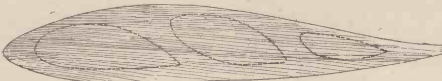
Fig. 42.—The form of the ribs. Fret away portion within the dotted lines. This section is the well-known R.A.F.34.
