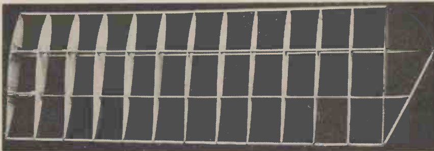
Fig. 39.—The right-hand main plane.
