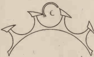
Fig. 8.—Showing the cylinder escapement.
