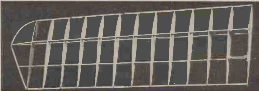
Fig. 40.—The left-hand main plane.
